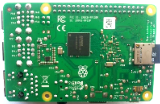
Figure 5. Raspberry Pi with SD Card inserted
